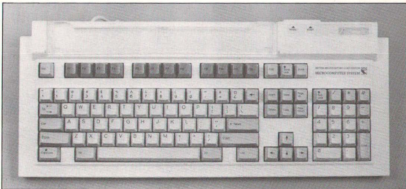
The keyboard features LEDs beneath the keys and 12 function keys. The mouse plugs into a port in the top right-hand corner
